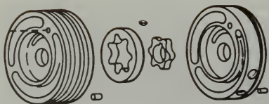
FIGURE 6-25. Typical gerotor pumping elements.
